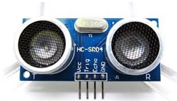
Figure 3: HCSR04 ULTRASONIC SENSOR
