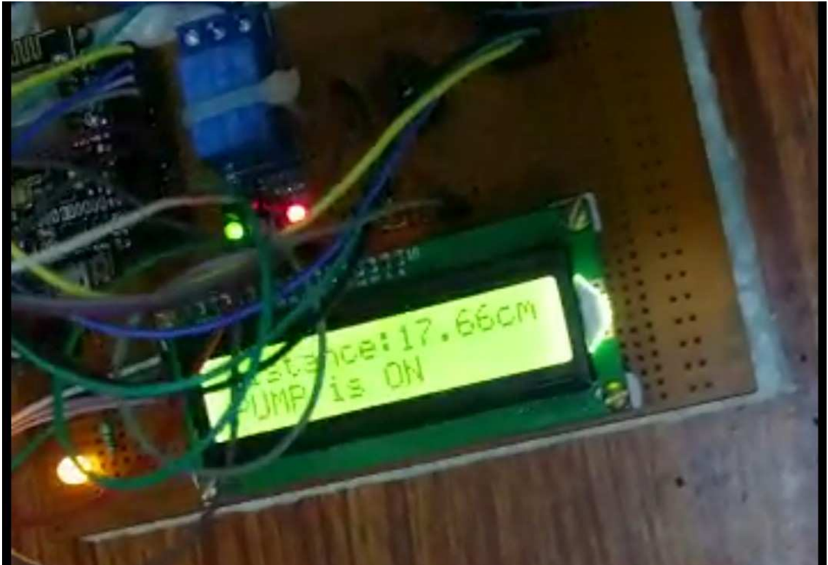
Fig 19. LCD Display displaying the distance
