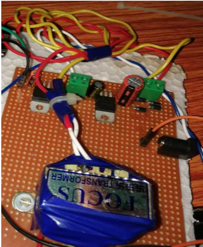
Fig 16. 5V Supply Circuit
