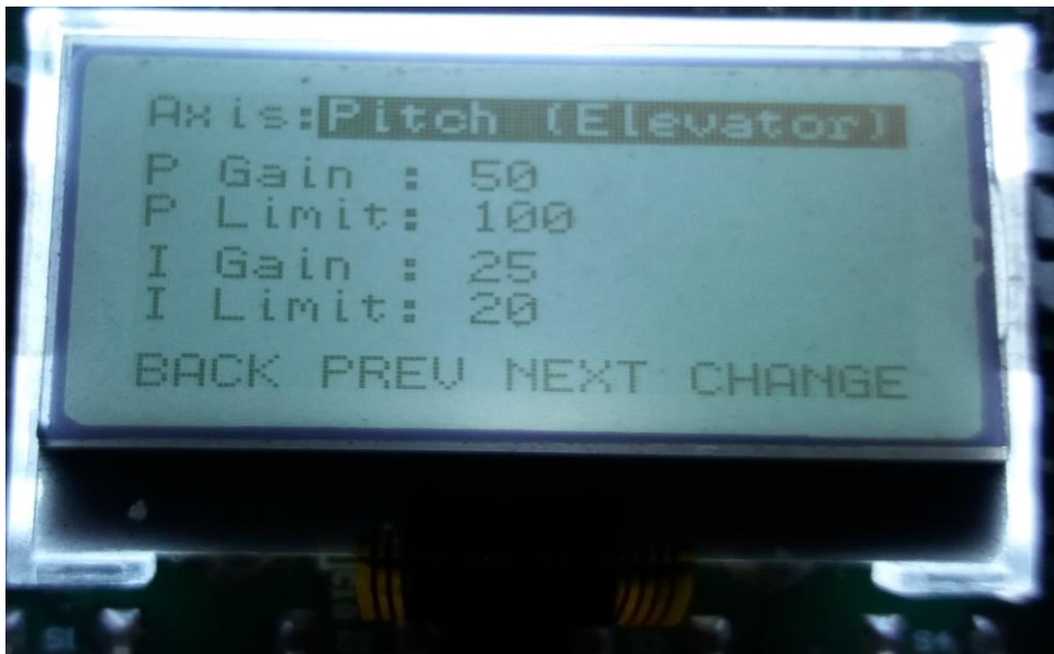
Fig. 4.3 Inside the PI Editor Menu and adjusting the Pitch Axis PI values for Stable Flight
