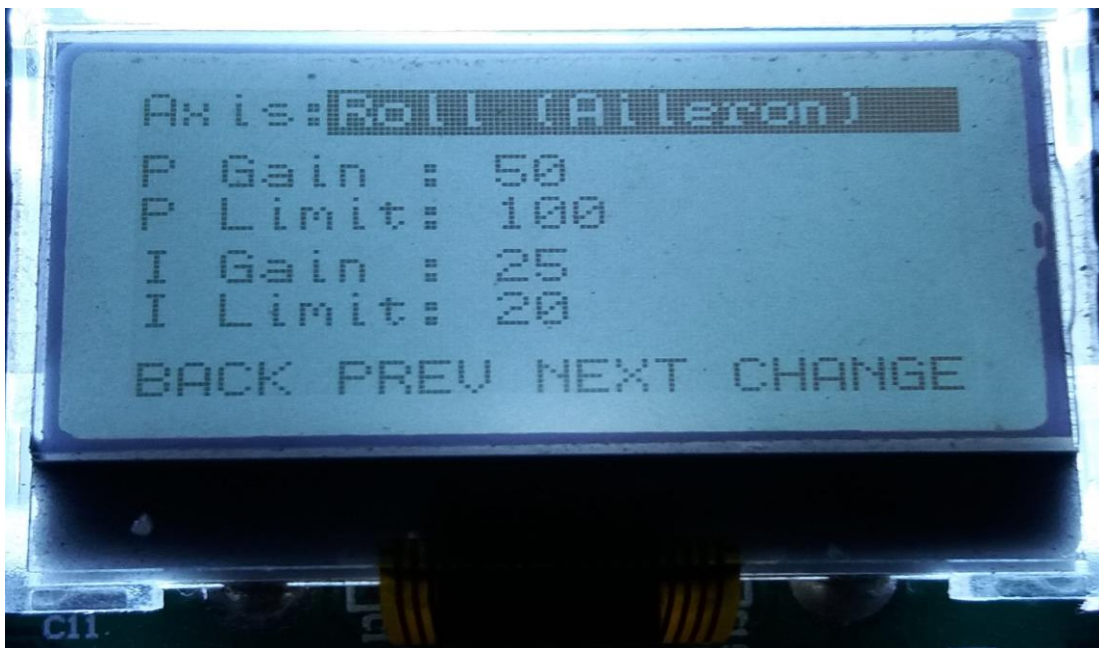
Fig. 4.2 Inside the PI Editor Menu and adjusting the Aileron Axis PI values for Stable Flight
