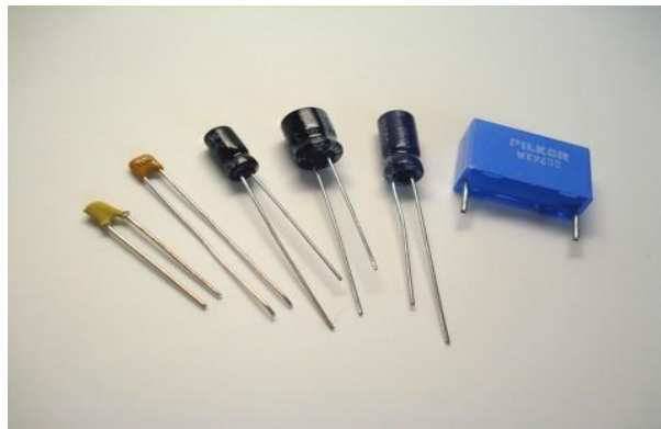
Figure 12: Types of capacitors
