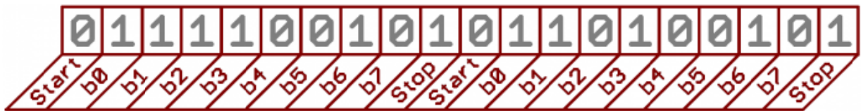
Figure 8: 9600 baud rate bit pattern
