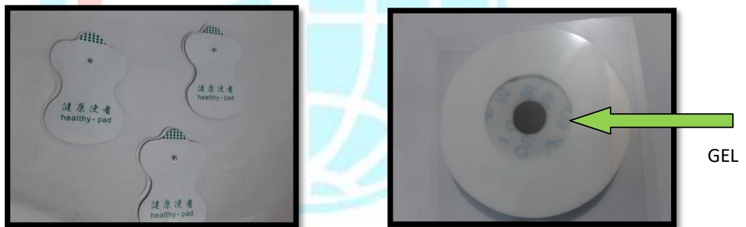
Fig.6a & 6b: Lead Electrodes and conducting gel
