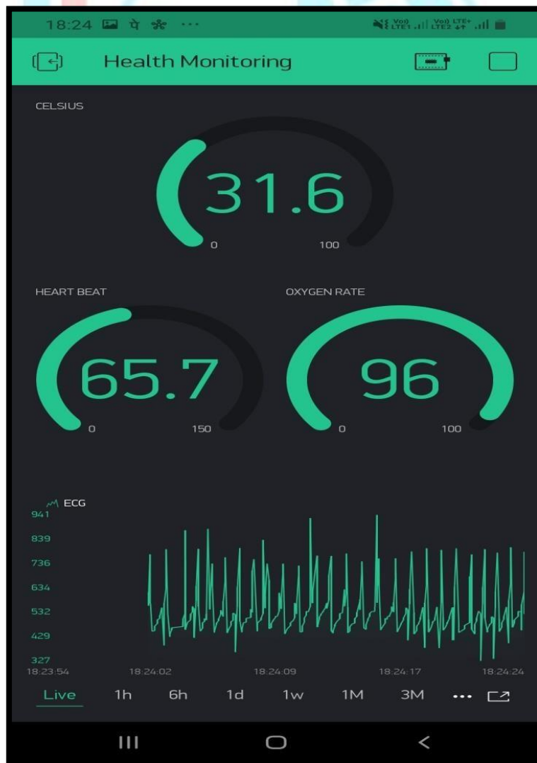
Fig.20: Measured body parameters displayed remotely on Blynk App
