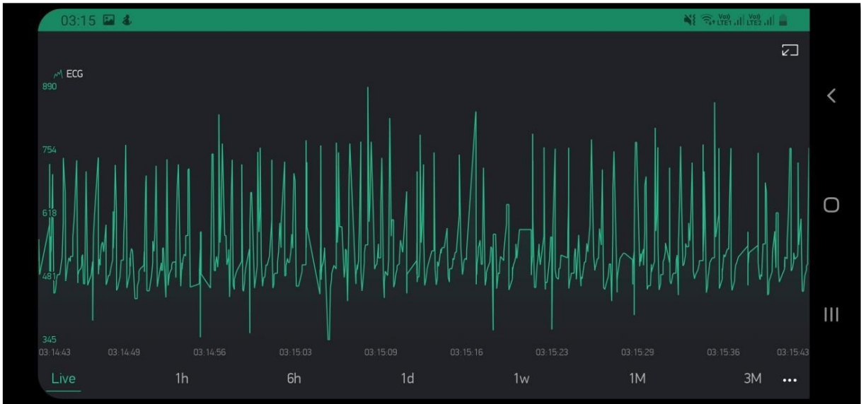
Fig.21: The ECG visualized separately on Blynk
