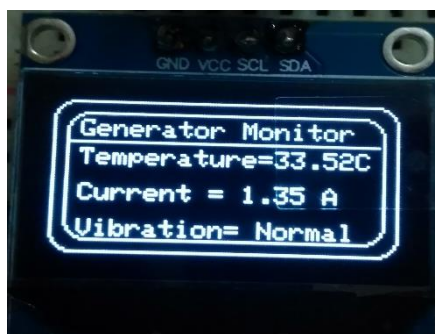
Figure 21: Some normal readings during operation
