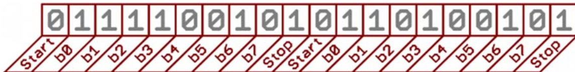
Figure 3: 9600 baud rate bit pattern
