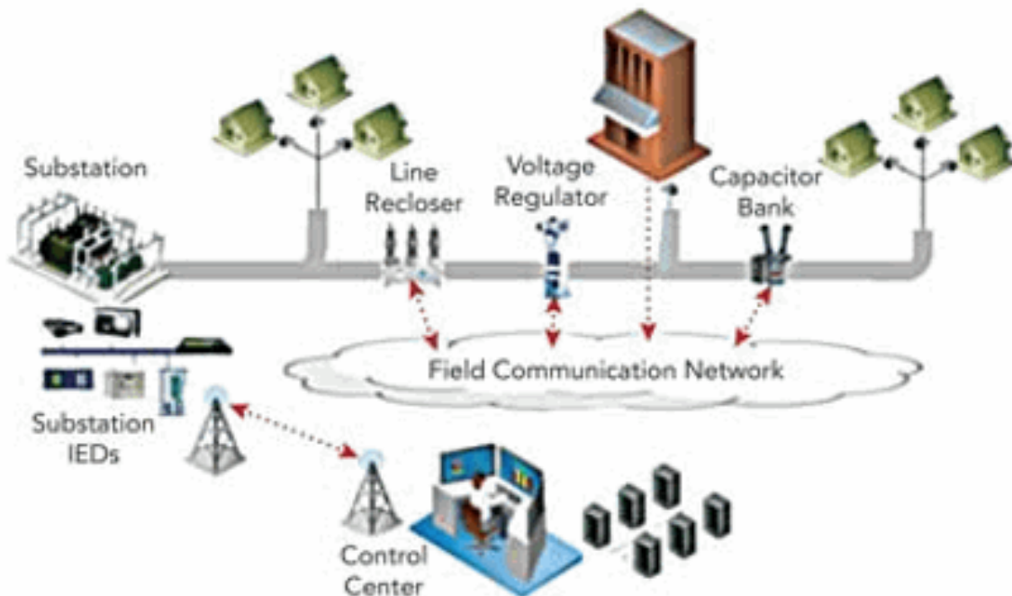
Figure 2.6: Typical Distribution Automation system at smart grid
