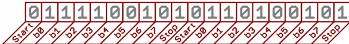
Figure 3: 9600 baud rate bit pattern
