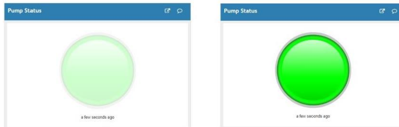
Fig. 22 Pump automatically gets on when the soil moisture content is below the threshold level.
