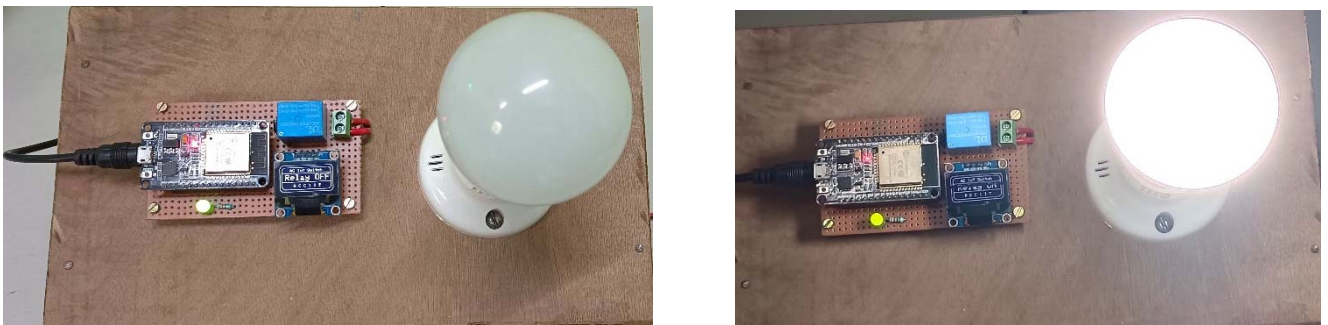
Figure 13: Load is switch off and switch on condition
