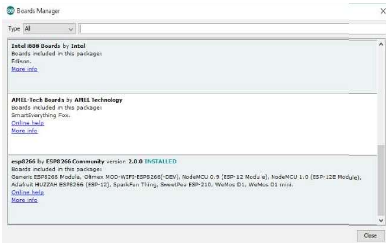
Figure 10: ESP 8266 board installation in Arduino
