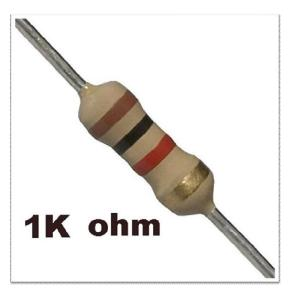
**Construction and Characteristics:** 1k-ohm resistors are typically made of a cylindrical ceramic or carbon composition material with metal leads extending from each end. The resistance value of 1k ohm indicates that when a voltage of 1 volt is applied across the resistor, it will allow acurrent of 1 milliampere toflowthroughit, according to 0 hm's Law (V=IR).
